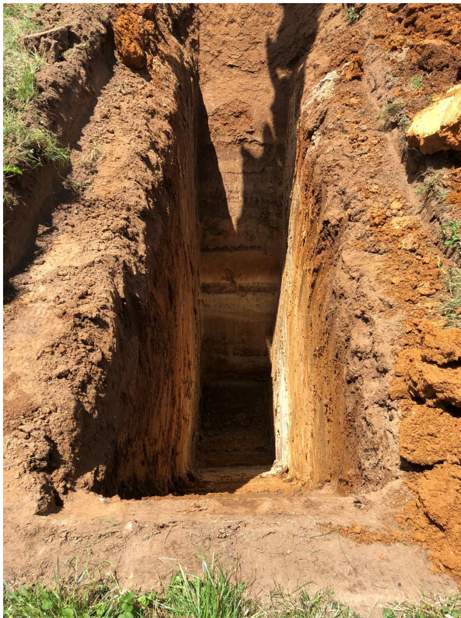
TP07 – TEST PIT EXCAVATION
