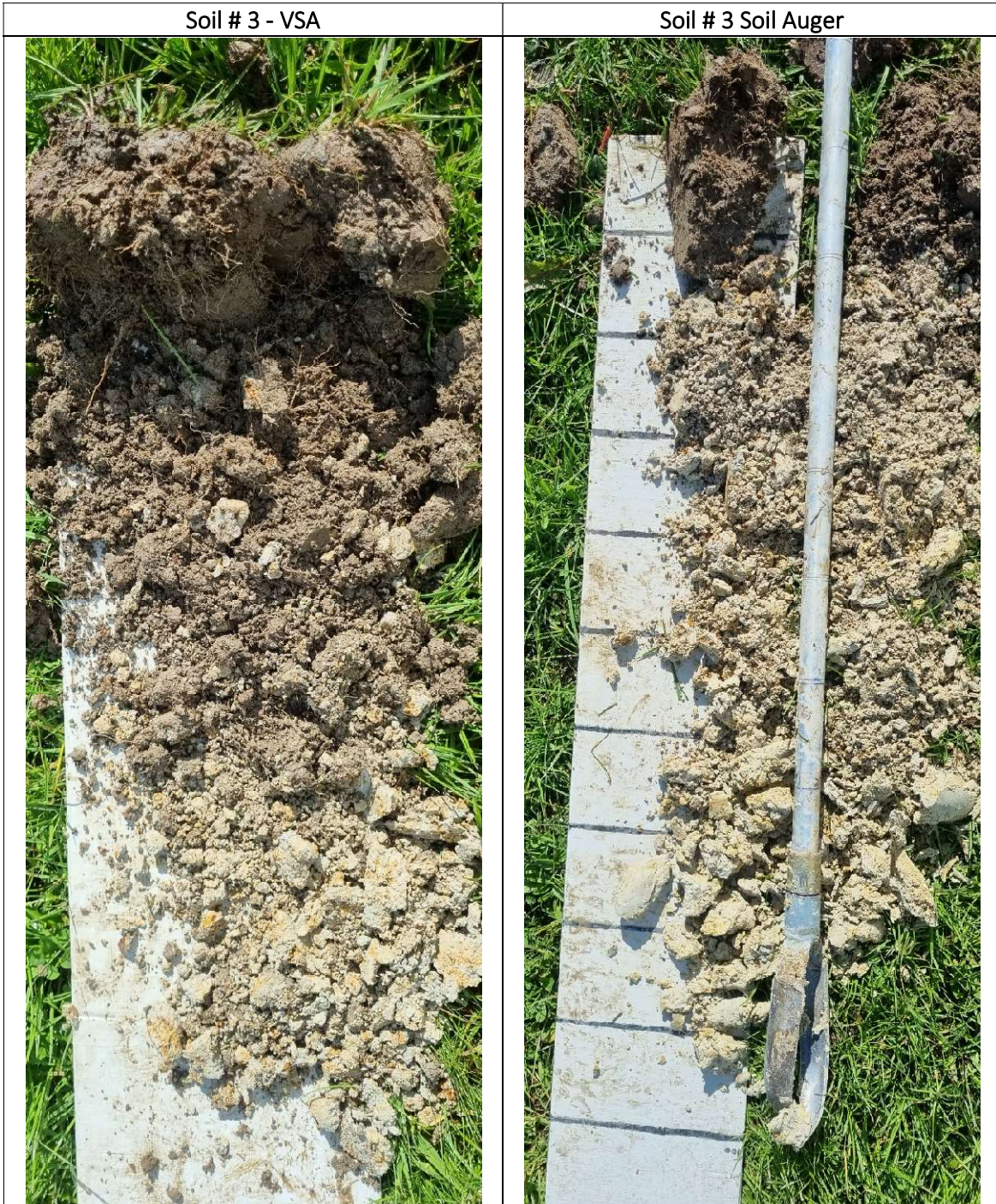
Figure 7c: Photos of soil auger observations
