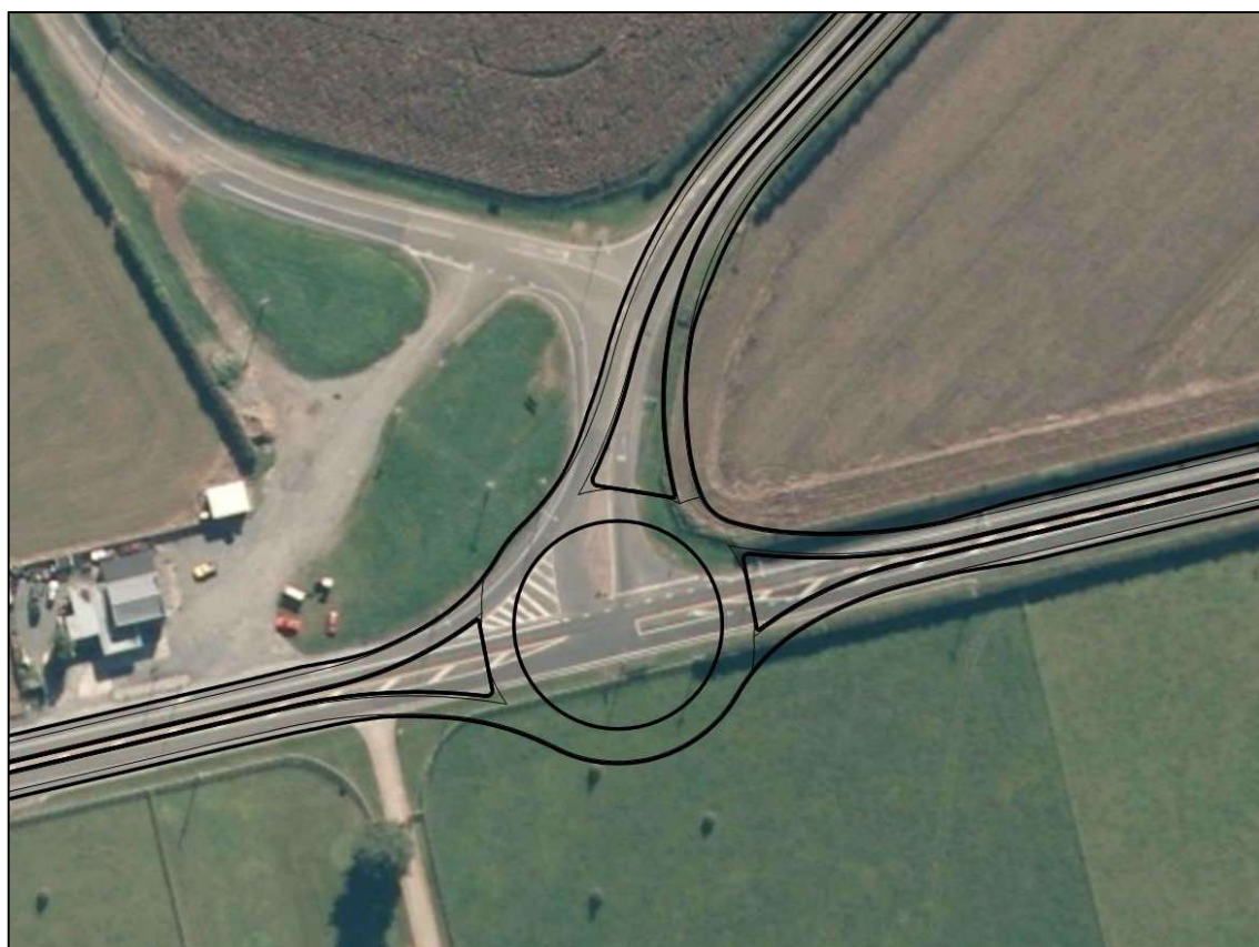
Figure 1: Schematic Design for Roundabout at SH 29 / Hopkins Road Intersection (image source: LINZ, 2019)
